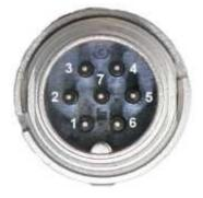
Pole diagram, contact side plug
