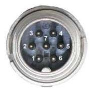
Pole diagram, contact side plug
